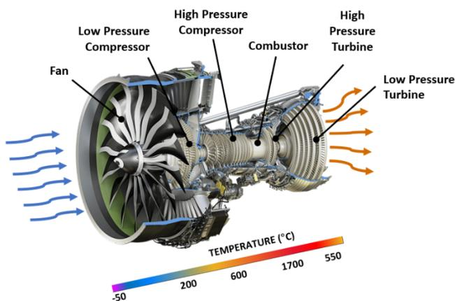
Figure 1. Cutaway view of a GE9X commercial aircraft engine<sup>4</sup> showing variation of temperature and pressure through the airflow path.
