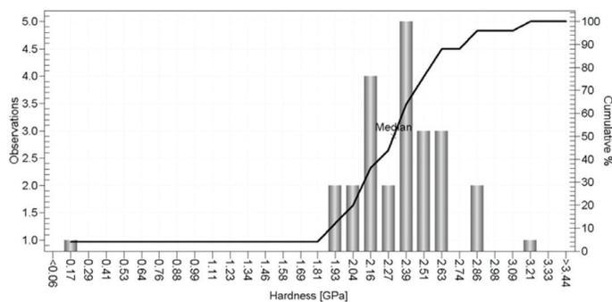
**Figure 3. Histogram of one set of 25 indents on sample B'. The median is 2.37 GPa; The mean (2.31 GPa) is affected by one aberrant indent (H = 0.17 GPa). Histogram is automatically generated by NanoSuite or InView software.**
